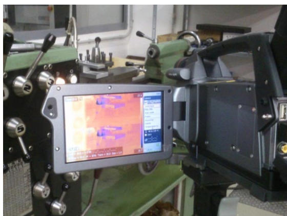
Fig. 4. Scanning device by TC Flir 660
