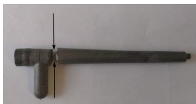
Fig. 4. The crack of the runner system detected for the feedstock E
