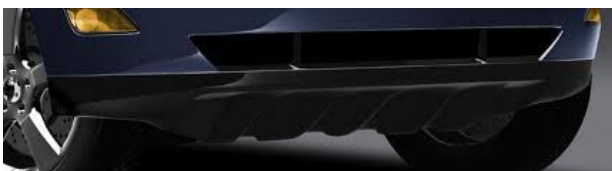
Fig. 1. Underbody shield made from LGFPP (provided by Styron)
