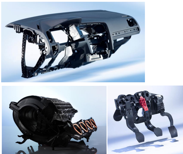
Fig. 2. Some structural PP application: VW Golf VII dashboard carrier made of expanded 20% short-glass fibre PP compound Xmod™ GE277AI (upper); air intake manifold - 35% short glass fiber PP Xmod™ GB306SAF (bottom left); pedal carrier made of 30% short glass fibre PP compound Xmod™ GD301FE (bottom right). The figures are not in scale
