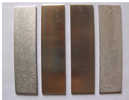
Fig. 5. Photographs of Al samples: (a) chemically cleaned Al sample, (b) pp-HMDSO sample, (c) pp-HMDSO sample after salt test, (d) chemically cleaned Al sample after salt test
