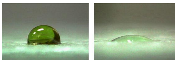
Fig. 5. Snapshots of drops (diiodomethane) before (left) and after (right) treatment
