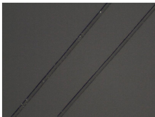
Fig. 6. Stereo microscope image of as-received untreated fibres
