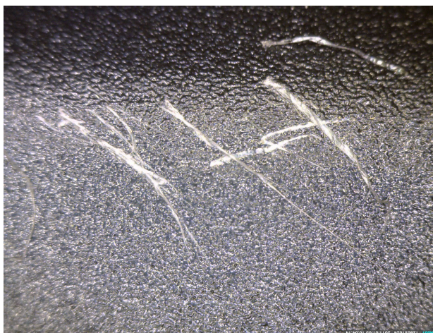
Fig. 4. Picture of a defect: white fibers coming out from a black car interior cover
