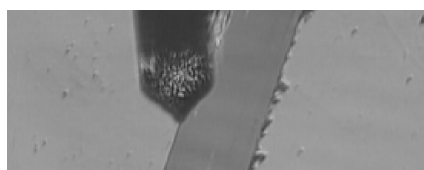
Fig. 2. The xerogel layer on glass with the scratch (50 μm wide) and with the AFM cantilever above the measured edge
