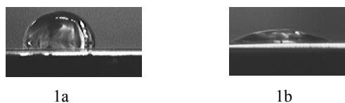
Fig. 1. A drop of water on the PP film before (1a) and after (1b) plasma treatment
