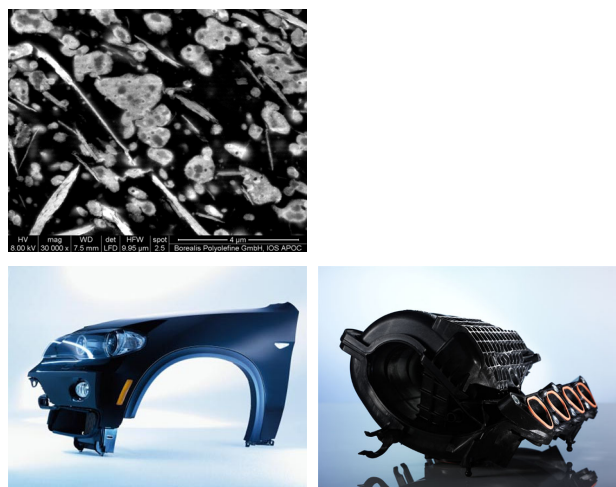
Fig. 1. Top : electron microscopy micrograph of the morphology of heterophasic mineral filled PP after RUO 4 staining; Bottom left : Fender Application for BMW X5 (mineral filled iPP compound Daplen TM EF341AE); Bottom right : Air Intake Manifold (glass-fibre filled iPP compound XMOD TM GB306SAF)
