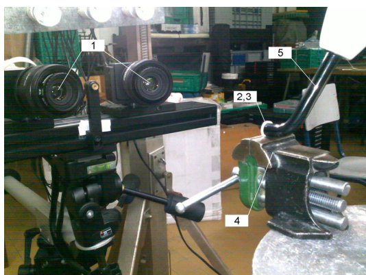
Fig. 2. Experimental setup. 1 – Cameras; 2 – Teflon mold; 3 – Sample; 4 – Sample holder; 5 – Light curing unit
