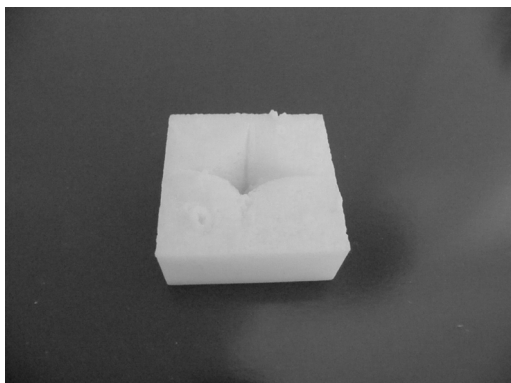
Fig. 3. Replication of the specimen surface using the rapid prototyping technique
