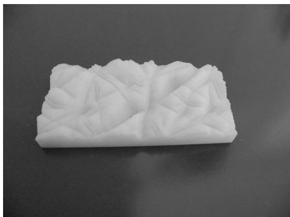
Fig. 5. 3D replication of the surface structure of the specimen created by rapid prototyping technique
