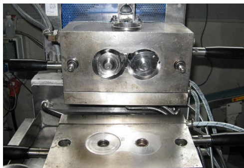
Fig. 2. Internal mixer, used to accomplish the mechanic-chemical method of devulcanization
