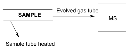
Fig. 4. Schematic presentation of a the EGA analysis
