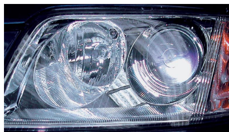
Scheme 7. Head Light Element made from Polycarbonate requires high level of UV- and heat stabilization
