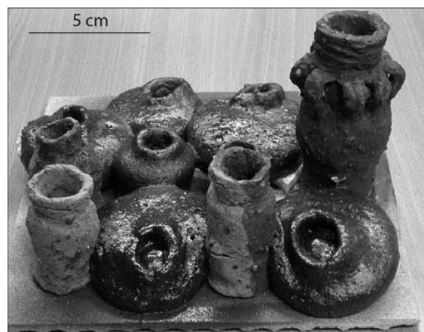
Fig. 4. Experimental firing of the Loštice pottery miniature replicas. The collapsed vessels were made of loess soil
