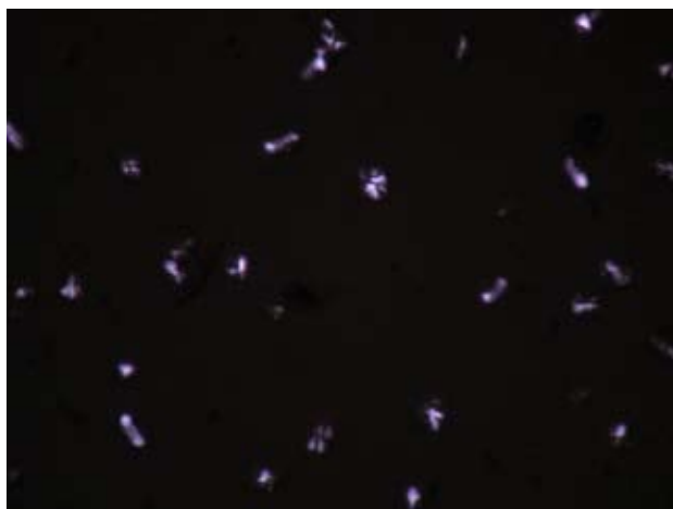
Fig. 1. The POM micrograph of the HDPE crystallization early stage
