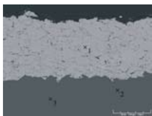
Fig. 1. The cross-sectional SEM image of Al substrate coated by Ni in as-received state
