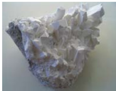
Fig. 2. Borax \text{Na}_2\text{B}_4\text{O}_7 \cdot 10\text{H}_2\text{O} i.e. Sodium tetraborate. It is applied in different industry: metallurgy, glass industry, ceramic industry and in some pulp mill
