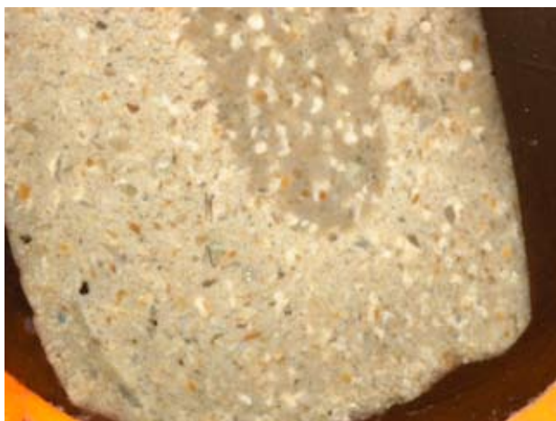
Fig. 6. Image in polarized light of thin section of MDF composite containing 6 % of polymer after 7 days in moist atmosphere
