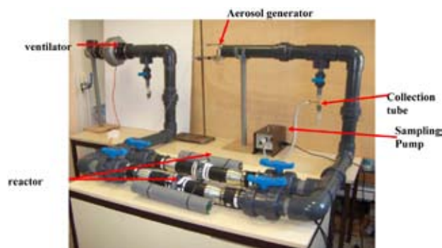
Fig. 8. Photos of experimental device used to test the efficiency of BUXAIR reactor against the avian influenza virus
