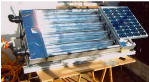
Fig. 6. AQUACAT autonomous solar photoreactor prototype for water potabilization
