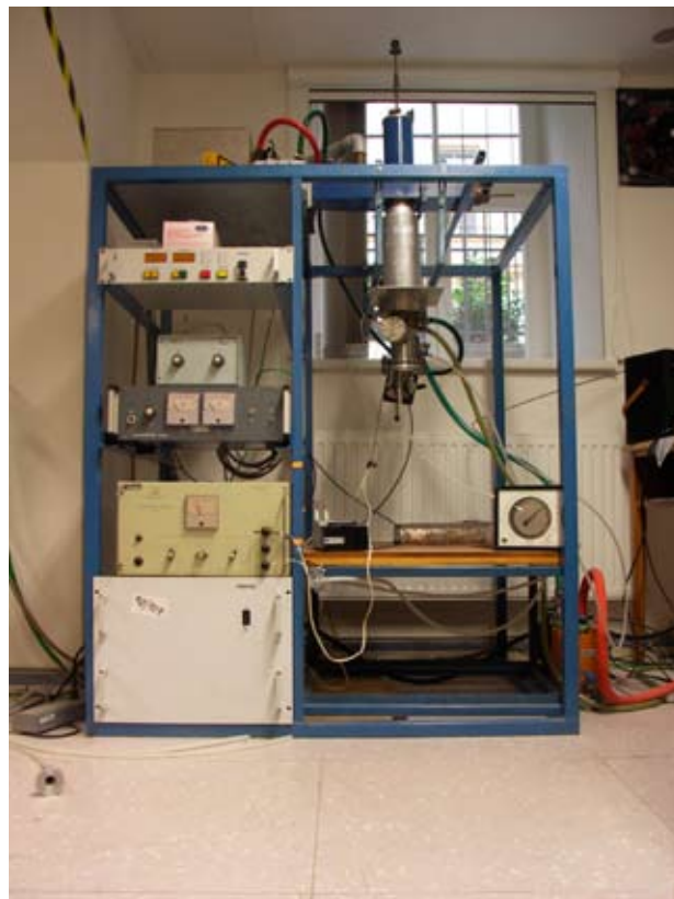
Fig. 2. Microwave ASTeX-type reactor used for UNCD deposition
