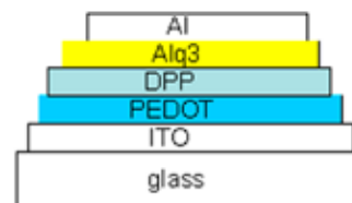
Fig. 1. Example of multilayered structure for electronic applications
