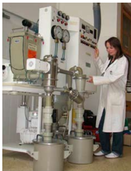
Fig. 5. Pilot plant air classifier
