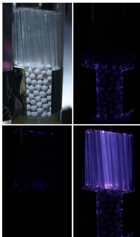
Fig. 3. Images of the discharge in capillaries [diameter 2 mm, length 3 mm] at different AC and DC applied voltages in ambient air: (top left) the reactor, (top right) barrier discharge [ U_{AC} = 16 kV, U_{DC} = 0 kV], (bottom left) corona discharge [ U_{AC} = 0 kV, U_{DC} = -20 kV], (bottom right) sliding discharge [ U_{AC} = 15 kV, U_{DC} = -16 kV]
