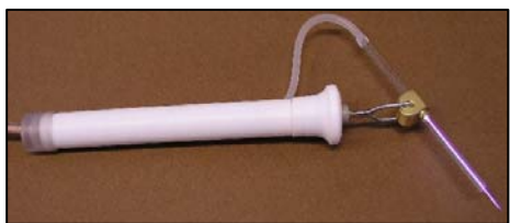
Fig. 1. Photograph of plasma pencil
