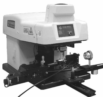
Fig. 1. UP 266 MACRO Laser Ablation System modified for double-pulse LIBS measurements. The ablation chamber was replaced with sample holder; the second laser pulse was focused by side glass lens and the laser induced plasma emission was collected by fiber placed in the front part
