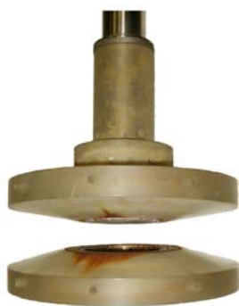
Fig. 15. Electrodes with a nozzles made from plexiglass
