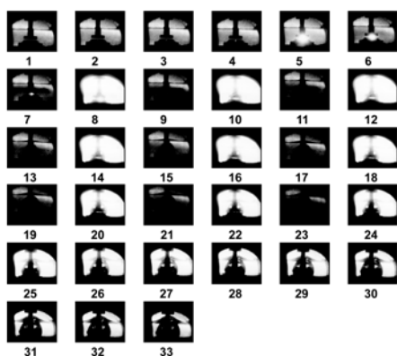
Fig. 11. Shadow photos of the discharge in a still service water. Frame exposure time – 25 \mu s. Time interval between frames 1 – 7, 24 – 33 is 50 \mu s. Between the others – 25 \mu s. Frames 1 – 7, 9, 11, 13, 15, 17, 19, 21 and 23 were taken with a help of blue light filter
