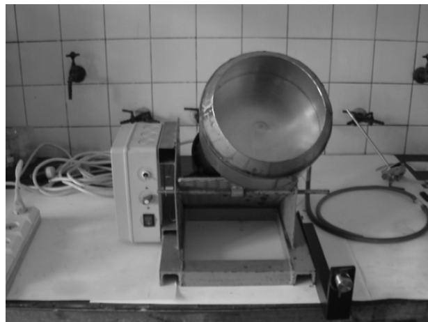
Fig. 1. Laboratory disc-type granulator
