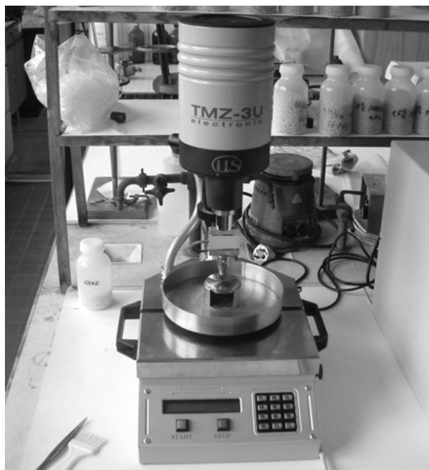
Fig. 2. Apparatus TMZ-3U for measuring strength
