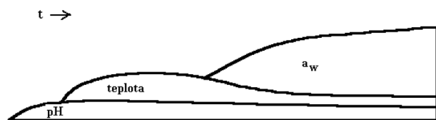
Fig. 1. Growth barriers of undesirable microorganisms and their development during processing of fermented meat products
