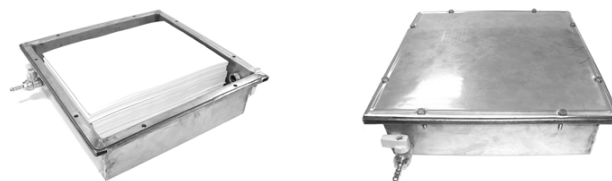
Fig. 1. Sealed reactor for aging of paper
